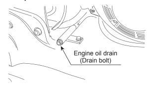
Figure 24. Draining Engine Oil
